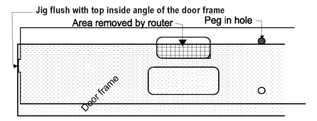
Remove all the pegs from the holes used when routing the door and insert them in the holes from the other side. Place the jig on the doorframe with the pegs against the vertical edge of the frame to which the hinge will be fitted, with the top of the jig hard against the inside top edge of the frame.
