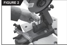
**Warning!** Always unplug the unit before changing grinding wheels, or when making any adjustments to the Sharpener.
