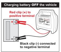
For batteries removed from the vehicle, place the black clip directly onto the negative terminal post (marked with a "-" symbol).
