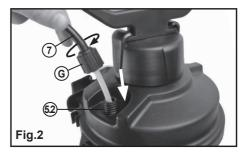
Insert the suction tubing of the hose (7) into the tank through the hose inlet (5.2). Screw the compression fitting (G) to secure the hose in place.
