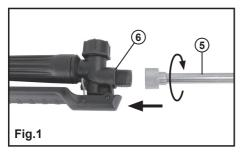
Screw the lance (5) onto the trigger assembly (6).
