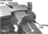
First pass the webbing strap though the fixed hook clip located on the side base of the tank, then through one of the locking clips (Fig.1).
