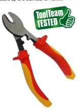
Length: 170mm (6<sup>3</sup>/4in) Cut Capacity: up to 10mm
